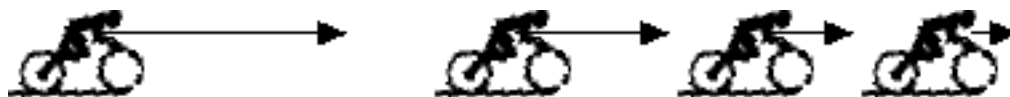
Figure 2: A motion diagram for a bike moving to the right with a decreasing speed.
