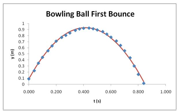
Graph 1: The position vs. time graph for the bowling ball's first bounce off of the trampoline. The subsequent bounces had similar shapes.
