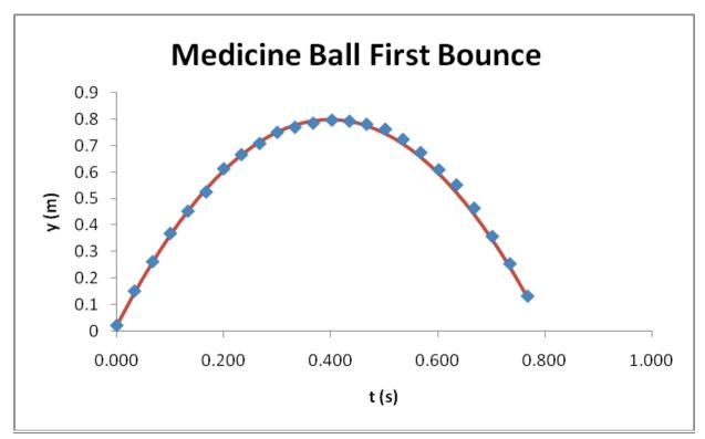
Graph 2: The position vs. time graph for the medicine ball's first bounce off of the trampoline. The subsequent bounces had similar shapes.
